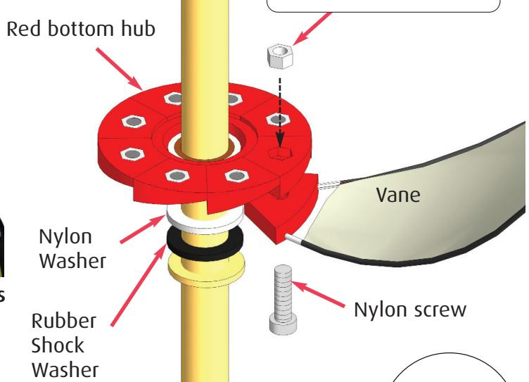
Do not overtighten nylon screws
