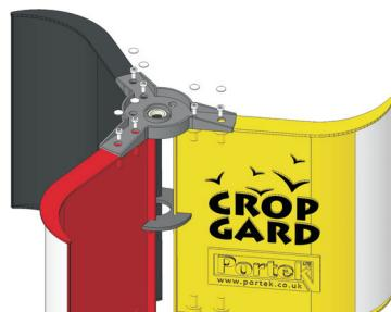
Locate the top bearing hub (C) in position on the blades (A). Use the self tapping screws (H) to fix securely. Press in the screw caps (I) to seal.
