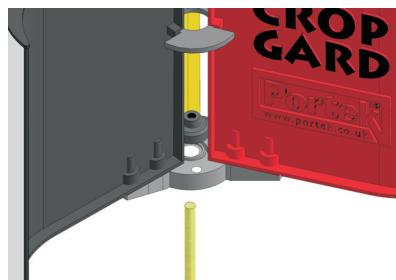
Insert the bottom rain cap (M) above the bottom hub (C) between the blades as shown in above.
