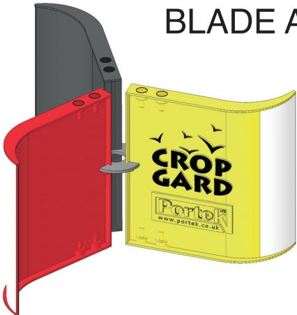
Place blades (A) on firm surface and locate them in position using the centre locating disc (B).
