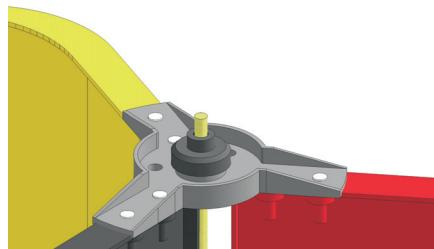
Take top rain cap (M) and push over solid top bar until it rests on the split pin.
