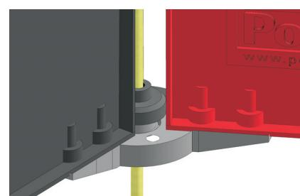
Ensure the bottom cap does not rub on the hub/blades keeping a 2 mm gap.
