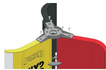
Turn over and repeat for bottom hub (C) (no caps to seal screws here).
