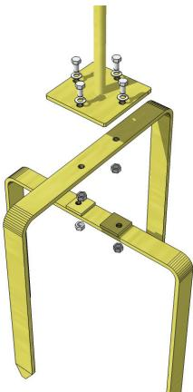
Bolt the two sets of ground forks (E) to the baseplate (D) using the setscrews, spacers and nuts (J, K & L).
